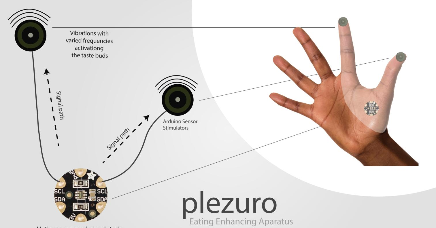
Motion sensor sends signals to the fingertip vibration caps as per movement of the fingers: closed and open
